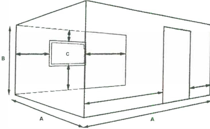
The first step is to measure all the walls from corner to corner (A), marking on your plan anything that projects into the room or recesses out. Measure the ceiling height (B) and clearly mark any changes in that height.
